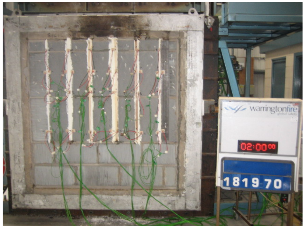
The unexposed face of the wall construction after 120 minutes of testing
