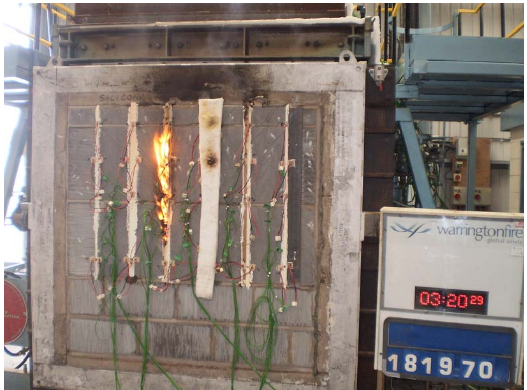
Integrity failure of Specimen I that occurred after 199 minutes of testing
