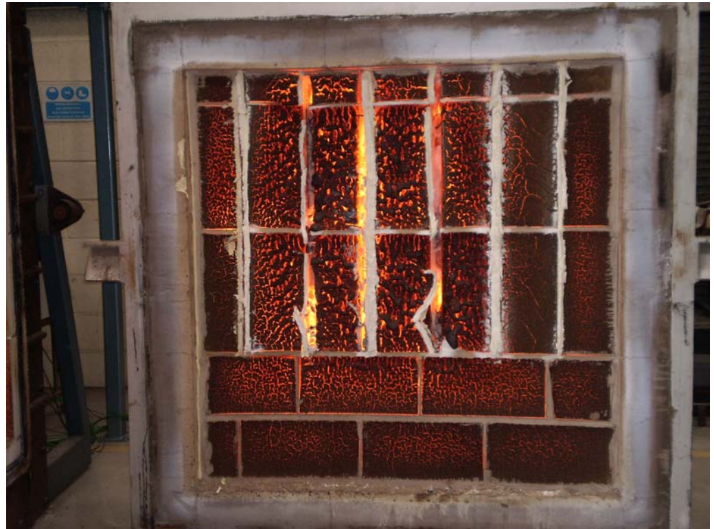
The exposed face of the wall construction immediately after testing
