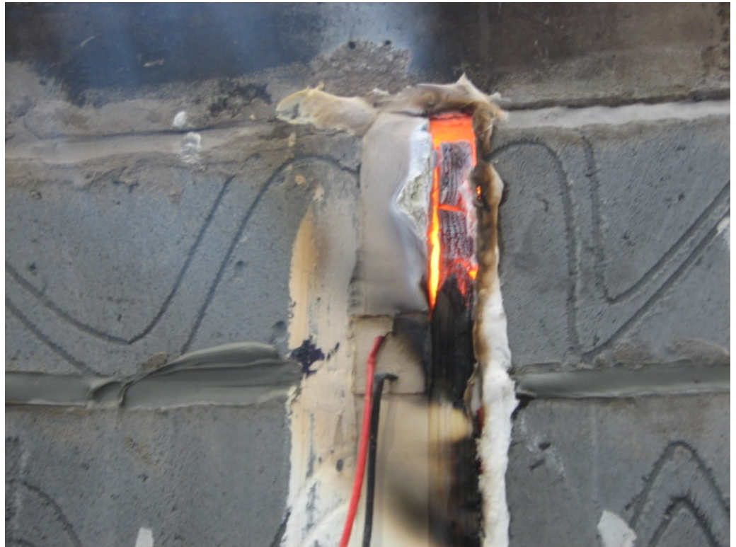
Integrity failure of Specimen J after 143 minutes of testing
