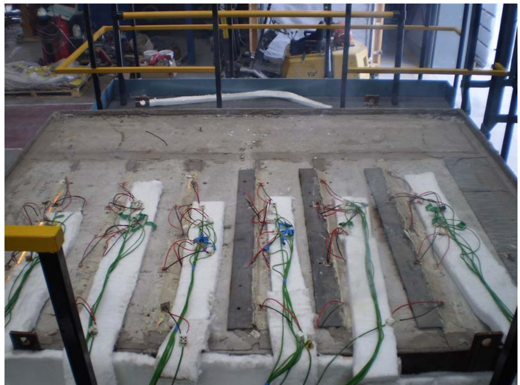
The unexposed face of the floor construction after 300 minutes of testing
