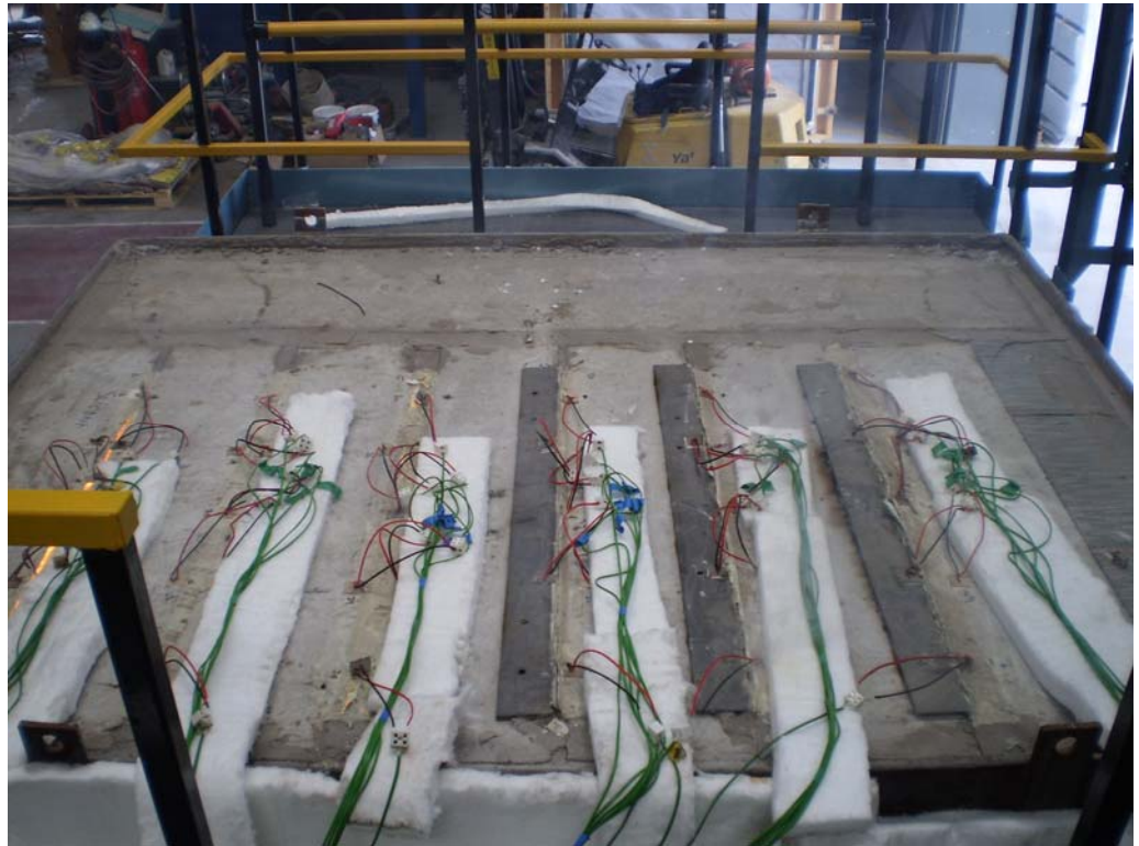
The unexposed face of the floor construction after 184 minutes of testing
